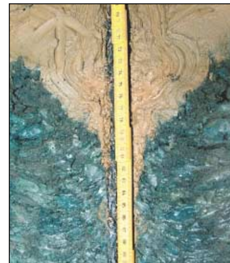
Selcore sample. Split liner showing the contact between the overburden clay and fragmented claystone.
