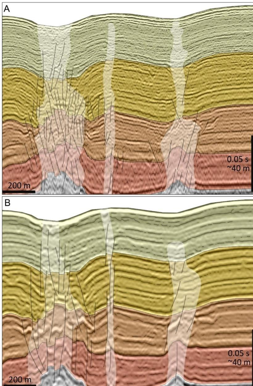
**Figure 3** Comparison between A) high frequency processing (bin size of 3.125x6.25m) and B) standard processing (bin size of 6.25x6.25m) along the same line within the P-Cable 3D cube acquired on the Vestnesa Ridge. Seismic data (courtesy of the Arctic University of Norway) imaged vertical chimney structures located below pockmarks associated with acoustic flares in the water column (Bünz et al., 2012).
