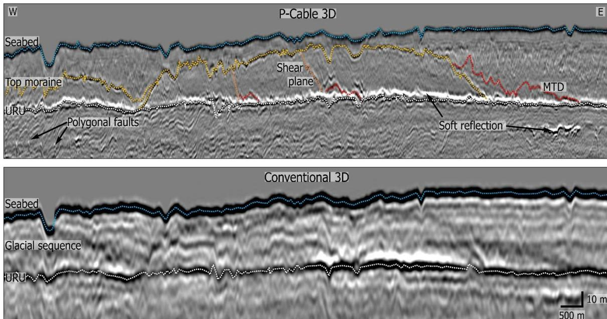
**Figure 2** Comparison of the first 100 m below the seafloor between P-Cable 3D (top) and conventional 3D (bottom) seismic data collected at the same location in the Barents Sea (seismic data courtesy of TGS). The figure (after Bellwald and Planke, 2018) shows that P-Cable data can image the internal structure of the glacial sequence, shallow stratigraphy, polygonal faults and soft reflections. Upper Regional Unconformity, MTD: Mass Transport Deposit.
