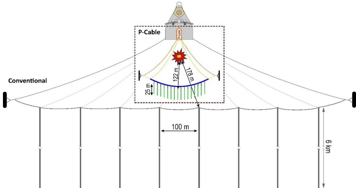
**Figure 1** Conventional and P-Cable 3D seismic acquisition setups at a similar scale. Arrows mark the streamer lengths and minimum offsets. Blue line represents the P-Cable cross-cable.
